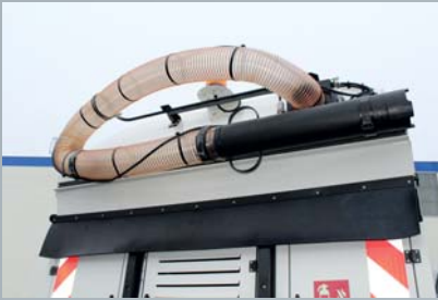
Manual suction hose at rear, DN 200
