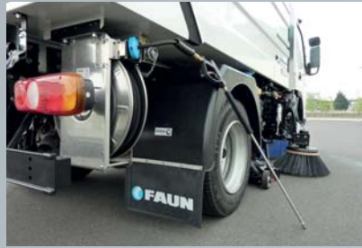
HP water pump with hose reel
